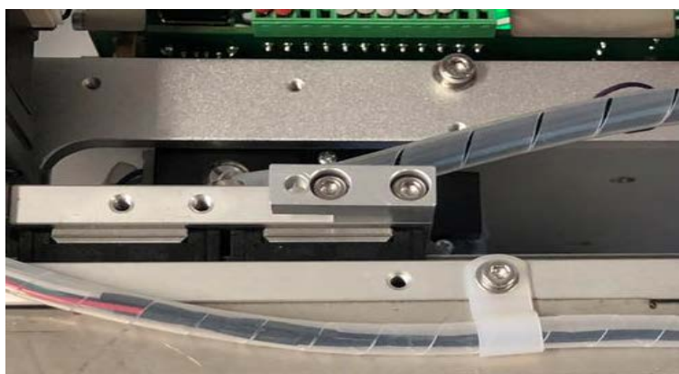
Figure 10 The fixing block fixed on the vertical plate
